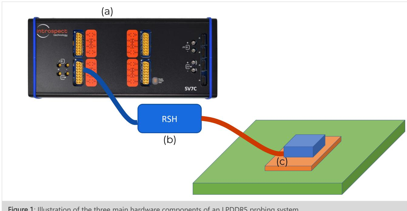
**Figure 1:** Illustration of the three main hardware components of an LPDDR5 probing system.
