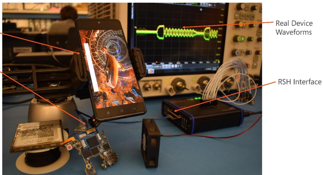
Figure 2: Illustration of the Remote Sampling Head connections.
